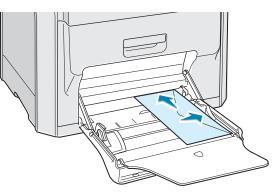
4 Pinch the paper width guide and slide it to the right to touch lightly against the edge of the stack without bending it.
